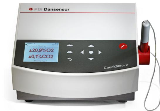
There are various measuring instruments on the market for measuring the oxygen and carbon dioxide contents in packaging. Samples are extracted with a small needle through a septum to ensure that the hole is closed after taking the sample. Prices range from 10,000 to 100,000 DKK.
