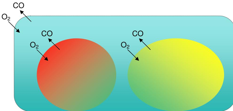
Packaging film for fruit and vegetables are never quite impervious to oxygen, carbon dioxide and water vapours. Even though the packaging film is welded quite tight, these gasses will be transported through the film (dissolved on the one side and liberated on the other). The rate depends on the type of plastic, the thickness of the film and the area, temperature and pressure differences of the gasses on each side of the film.
